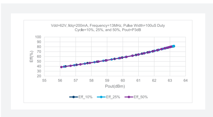
Fig. 10: (Swept Duty Cycle) drain efficiency (%) as a function of P OUT (dBm)
