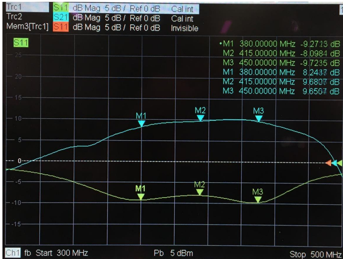
Figure 3 BLP9LA25S Low signal frequency sweep
